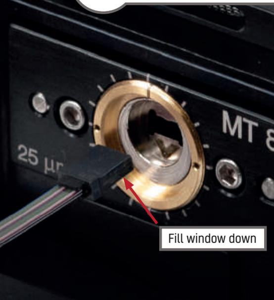
Hold the epoxied ferrule or connector at its base and carefully insert it into the Adapter Hole as far as it will go. For MT ferrules, the epoxy fill window must face down.
