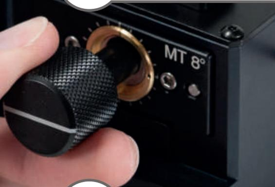
MT 0° and MT 8° ferrule adapter insert slots should be oriented horizontally with the arrow pointing down. For other adapter orientations, see User Information: Connector and Ferrule Adapters.
