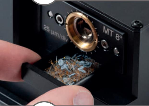
For non-vacuum models, periodically check the Waste Bin, and when necessary, safely dispose of its contents.
