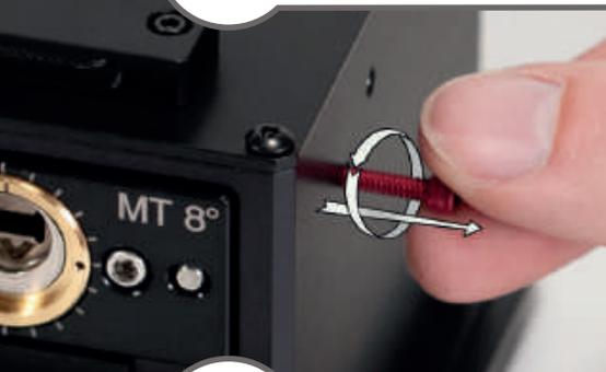
Re-install shipping screw if shipping or transporting the fibersect. Hand-tighten only.
